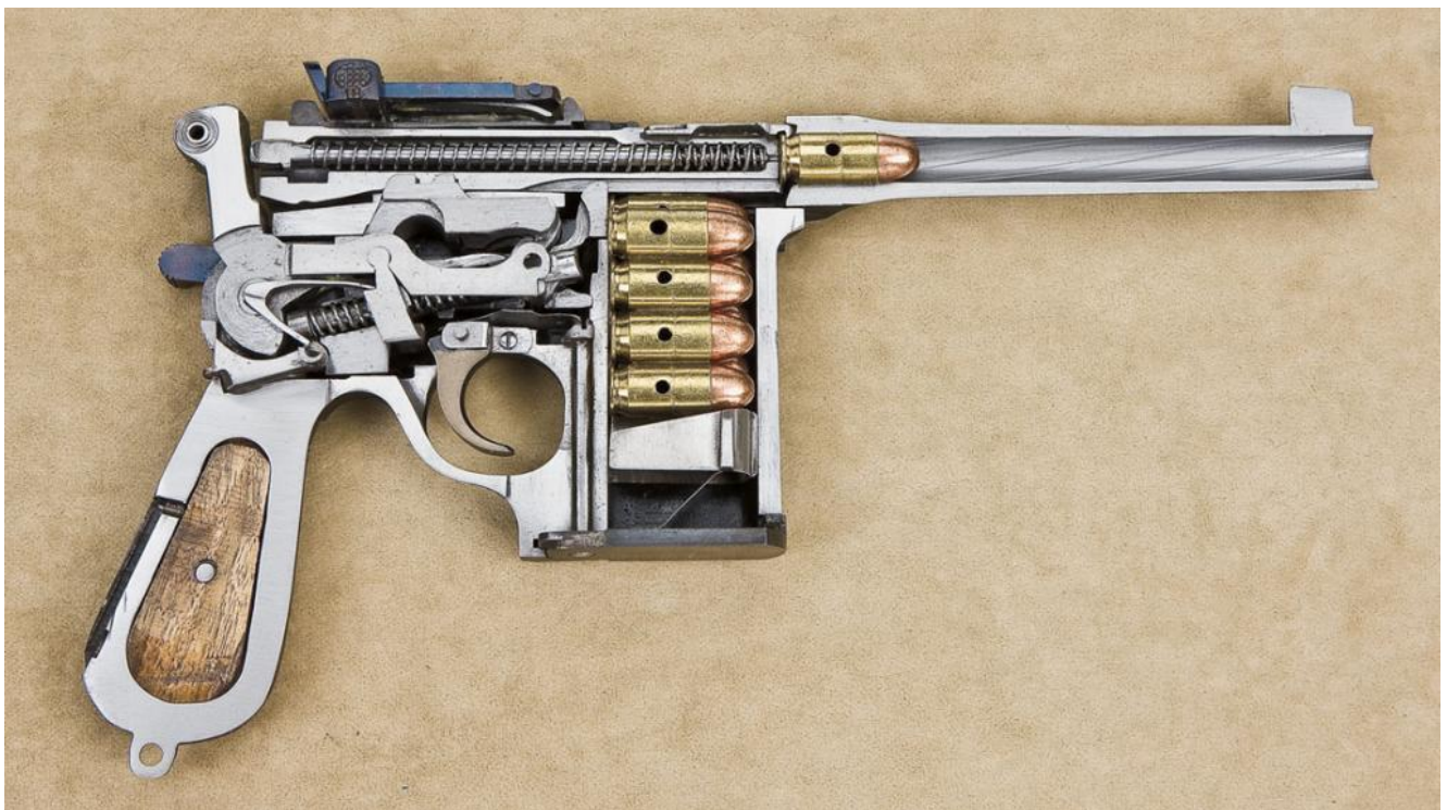
The Mauser C96, 7.63 & 9mm cut-away & loading strips
